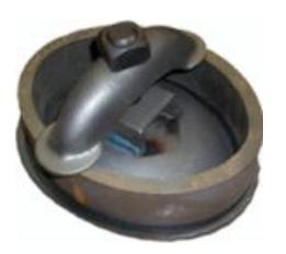
WORKING PRESSURE AS MENTIONED IS STAMPED ON PLATE, PLATES ARE FOR USE TO 650 DEGREE F UNDER ASME BOILER AND PRESSURE VESSEL CODE, PLATE MATERIAL IS SA516-70 OR SA285C, RING MATERIAL IS SAi06S OR SA106C
