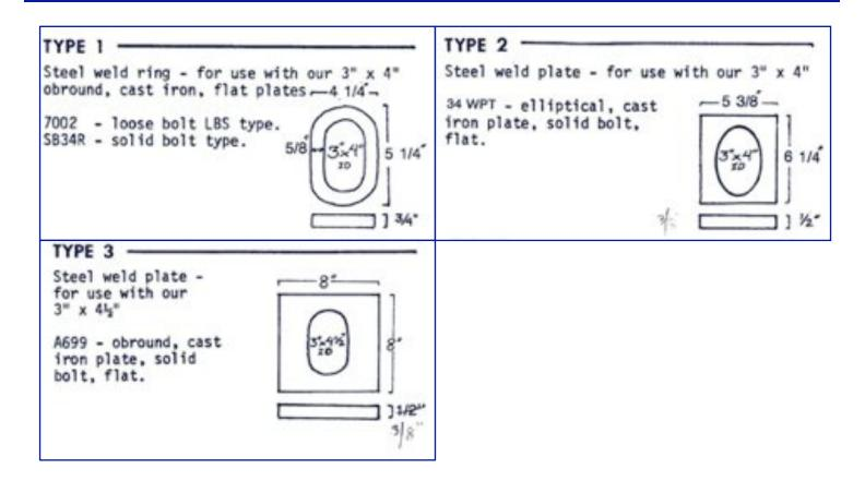
3" X 4"ELLIPTICAL INTEGRAL STUD TYPE CURVED PLATES, FORMED ON 4" AXIS ARE STOCKED; 9", 14", 15", 16", 18",24",27",31",42",48", AND 60" RADIUS, (18" TO 120" SHELL DIAMETER), 3" X 4" ELLIPTICAL WELD STUD TYPE CURVED PLATES ARE STOCKED: 9", 14", 15", AND 18" RADIUS,
